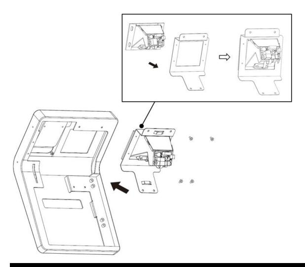
CF-3680 Scanner installation is Complete. Please Proceed to Step\_20 for A7 installation or/and <u>Step 13</u> if for Floor-type Application.
